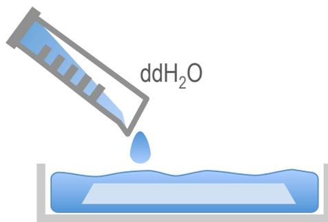
1. About 100ml of bidistilled water is added to the gel and heated in the microwave oven for 45 seconds. (avoid boiling). The box with the gel is then placed on a shaker for 3-5 min. Repeat twice this step with fresh water.
