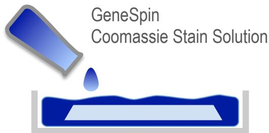
2. Cover the gel in the box with GeneSpin CS solution and heat in the microwave for 30 sec. without boiling. Place the box on a shaker for finishing the staining.
